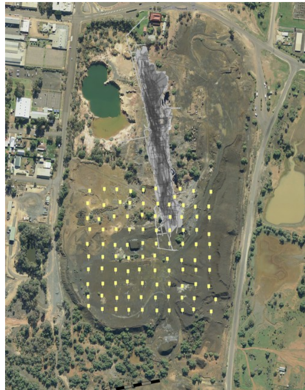
Figure 1: Locations of the seismic sensors relative to the suspected locations of the old workings.
